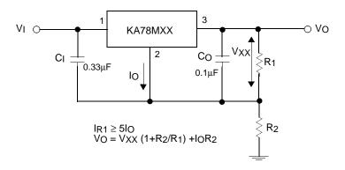
Figure 3. Circuit for Increasing Output Voltage
