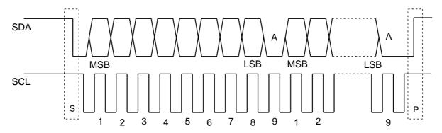
S; Start condition, a high to low transition of the SDA line while SCL is high P; Stop condition, a low to high transition of the SDA line while SCL is high A ; Acknownledge
