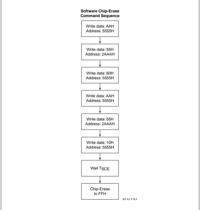
FIGURE 19: SOFTWARE CHIP-ERASE COMMAND CODES
