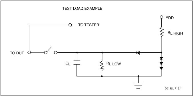
FIGURE 14: A TEST LOAD EXAMPLE
