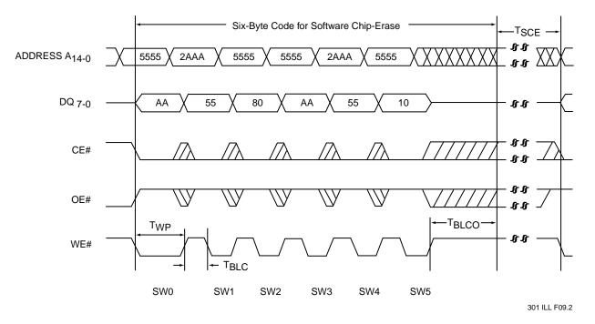
FIGURE 10: SOFTWARE CHIP-ERASE TIMING DIAGRAM
