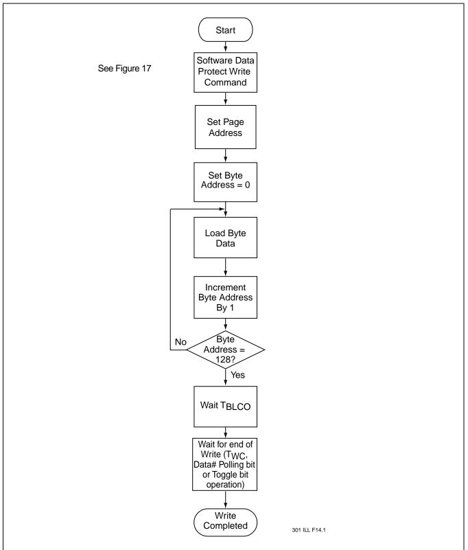
FIGURE 15: WRITE ALGORITHM
