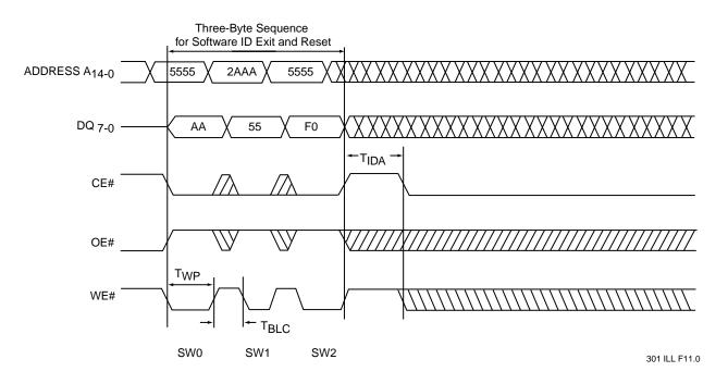
FIGURE 12: SOFTWARE ID EXIT AND RESET
