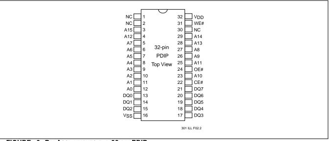
FIGURE 3: PIN ASSIGNMENTS FOR 32-PIN PDIP
