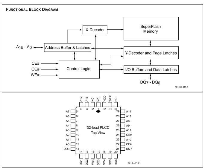
FIGURE 1: PIN ASSIGNMENTS FOR 32-LEAD PLCC
