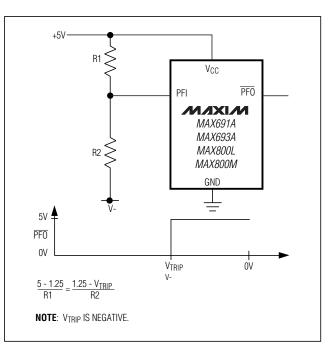
Figure 12. Monitoring a Negative Voltage
