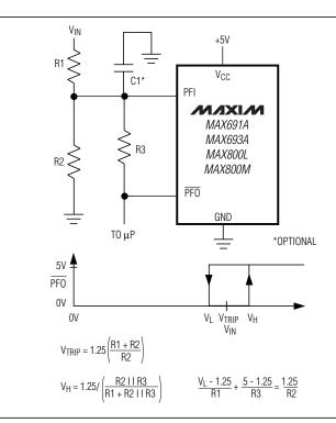
Figure 11. Adding Hysteresis to the Power-Fail Comparator
