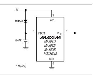
Figure 9. SuperCap or MaxCap on VBATT
