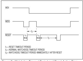
Figure 2. Watchdog Timeout Period and Reset Active Time
