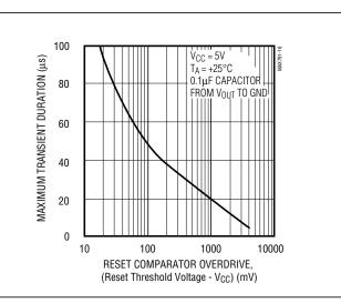
Figure 13. Maximum Transient Duration without Causing a Reset Pulse vs. Reset Comparator Overdrive
