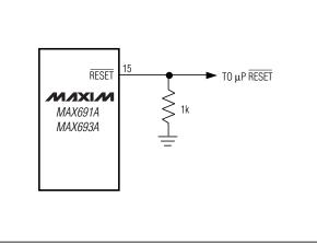
Figure 1. Adding an external pull-down resistor ensures  $\overrightarrow{RESET}$  is valid with  $V_{CC}$  down to GND.
