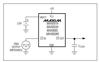
Figure 6. CE Propagation Delay Test Circuit
