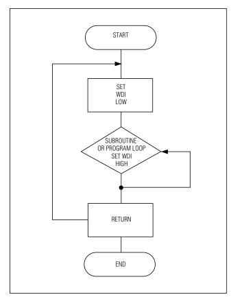
Figure 14. Watchdog Flow Diagram
