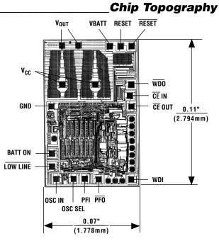
TRANSISTOR COUNT: 729 SUBSTRATE CONNECTED TO VOUT
