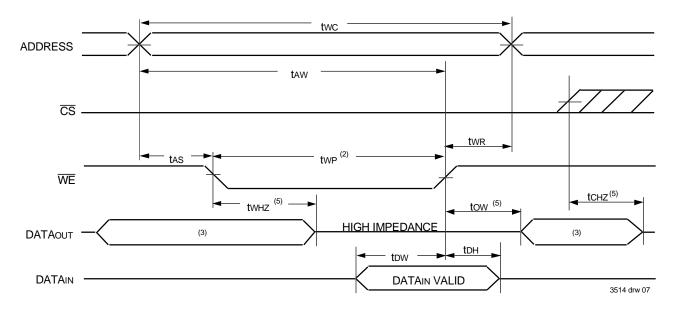
Timing Waveform of Write Cycle No. 2 (CS Controlled Timing)<sup>(1,4)</sup>
