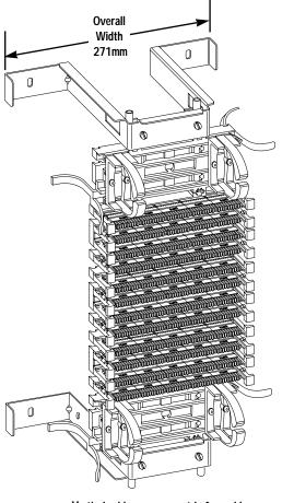
Vertical cable management is formed by butting ring runs in adjacent columns.
