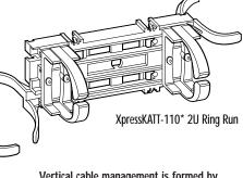
Vertical cable management is formed by butting ring runs in adjacent columns.
