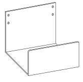
36.C0084 PDS Wall Mt. Frame Drip Tray 133mm x 222mm x 108mm Shipping Weight: 880g
