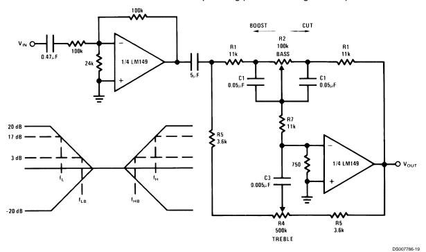
$$\begin{split} &V_S=\pm 15\text{V},\ V_{OUT(MAX)}=9.1\ V_{RMS},\\ &f_{MAX}=20\ \text{kHz},\ THD \leq 1\%\\ &\text{Duplicate the above circuit for stereo} \end{split}$$
