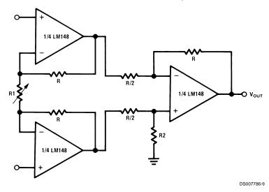
$$V_{OUT} = 2 \bigg( \frac{2R}{R1} + 1 \bigg) \text{ , } V_{\overline{S}} - 3V \leq V_{IN\,CM} \leq {V_S}^+ - 3V,$$
