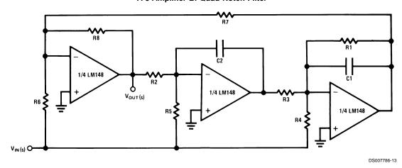
$$Q = \sqrt{\frac{R8}{R7}} \times \frac{R1C1}{\sqrt{R3C2R2C1}} \,, \ \, f_0 = \frac{1}{2\pi} \sqrt{\frac{R8}{R7}} \times \frac{1}{\sqrt{R2R3C1C2}} \,, \ \, f_{NOTCH} = \frac{1}{2\pi} \sqrt{\frac{R6}{R3R5R7C1C2}}$$
