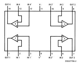
Top View Order Number LM148J, LM148J/883, LM149J/883, LM248J, LM348M, or LM348N See NS Package Number J14A, M14A or N14A LM148J is available per JM38510/11001
