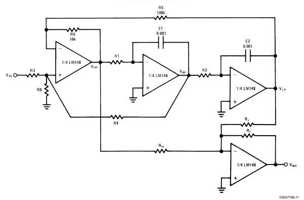
Tune Q through R0, For predictable results:  $f_Q \ Q \le 4 \ x \ 10^4$  Use Band Pass output to tune for Q
