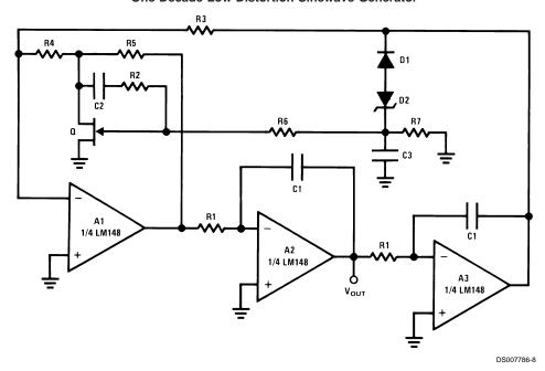
$$f = \frac{1}{2\pi R1C1} \times \sqrt{K}, \, K = \frac{R4R5}{R3} \left(\frac{1}{r_{DS}} + \frac{1}{R4} + \frac{1}{R5}\right), \quad r_{DS} \approx \frac{R_{ON}}{\left(1 - \frac{V_{GS}}{V_{D}}\right)^{1/2}} \label{eq:force_force}$$
