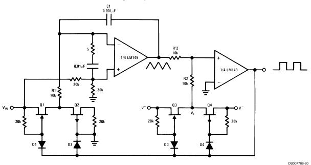
$$f = \frac{K \times V_{IN}}{8V^{+}C1R1} \,, \ K = R2/R'2 \,, \ \frac{2V_{I}}{K} \le 25V, \ V^{+} = V^{-}, \ V_{S} = \ \pm 15V$$
