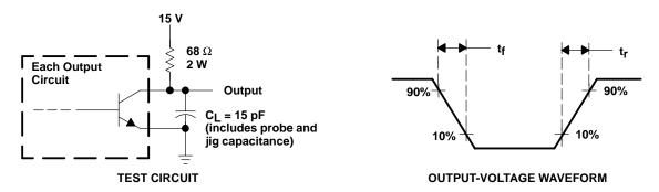
Figure 3. Common-Emitter Configuration
