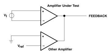
Figure 1. Amplifier-Characteristics Test Circuit
