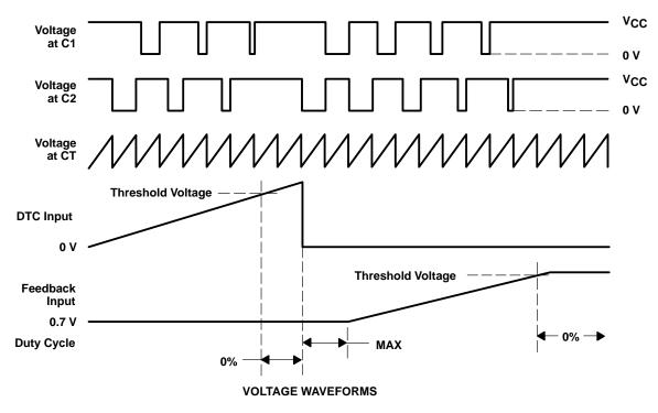
Figure 2. Operational Test Circuit and Waveforms
