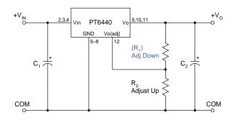
The values of  $(R_1)$  [adjust down], and  $R_2$  [adjust up], can also be calculated using the following formulas. Refer to Figure 1 and Table 2 for both the placement and value of the required resistor; either  $(R_1)$  or  $R_2$  as appropriate.
