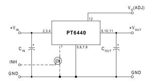
$C_{in}$  = Required 100 $\mu$ F electrolytic  $C_{out}$  = Required 330 $\mu$ F electrolytic
