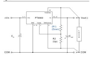
The respective values of (R1) [adjust down], and R2 [adjust up], can also be calculated using the following formulas.
