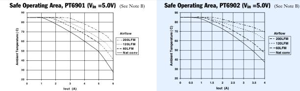
Note A: All data listed in the above graphs has been developed from actual products tested at 25°C. This data is considered typical data for the DC-DC Converter. Note B: SOA curves represent operating conditions at which internal components are at or below manufacturer's maximum operating temperatures
