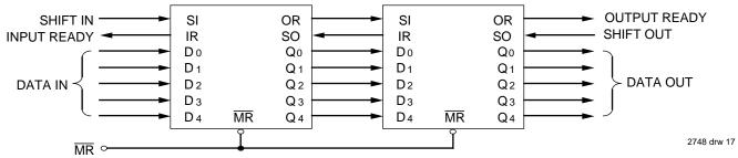
1. FIFOs can be easily cascaded to any desired depth. The handshaking and associated timing between the FIFOs are handled by the inherent timing of the devices.
