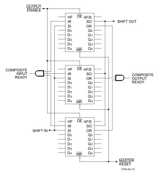
1. FIFOs are expandable in width. However, in forming wider words two external gates are required to generate composite Input and Output Ready flags. This requirement is due to the different fall-through times of the FIFOs.
