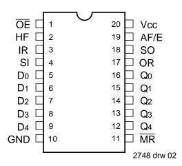
PLASTIC DIP (P20-1, order code: P) CERDIP (D20-1, order code: D) SOIC (SO20-2, order code: SO) TOP VIEW
