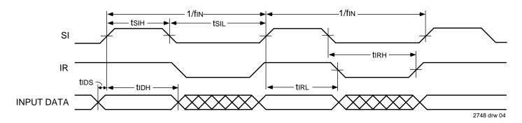
Figure 2. Input Timing
